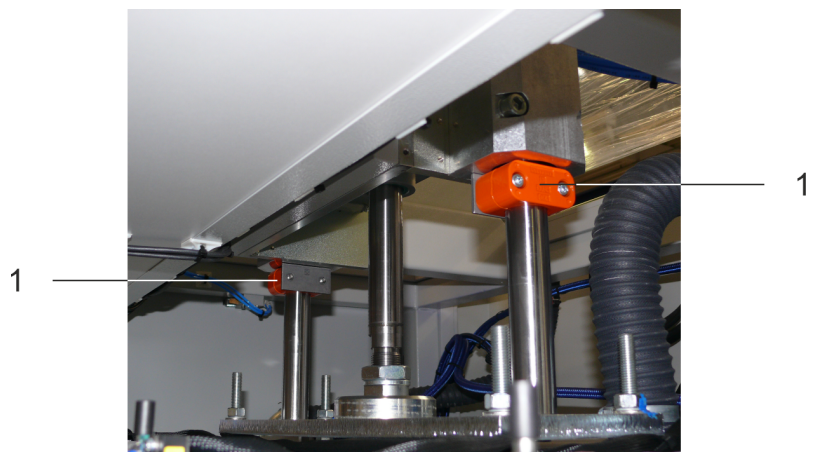
Fig. 7: Transport safeguard for upper buck guiding unit
